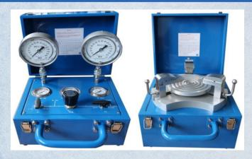
PTP-1A is a portable and robust machine for testing the opening pressure and sealing performance of pressure safety valves. It provides quick and efficient testing for a series of valves ONSITE.
